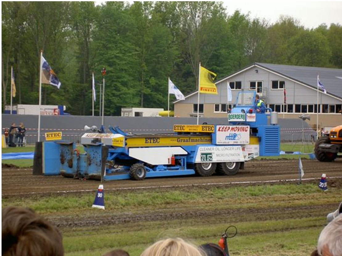
The same Sledge before being modified. Note the difference in the angle of the box rails. (source ETPC web site).
